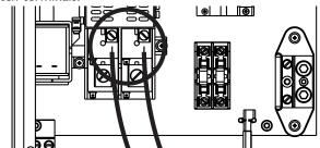
Slide one current transformer (CT) over each generator power supply lead and reconnect generator power supply leads to contactor terminals.
